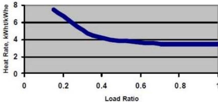
Figure 6 Heat rate versus load ratio for GT model 9171E gas turbine (ambient Temperature = 20°C)
