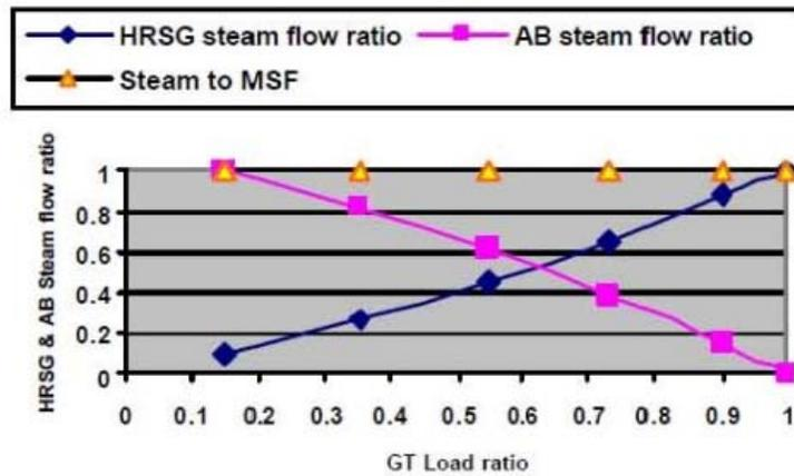
Figure 2 HRSG and AB steam flow ratios for various GT load ratios
