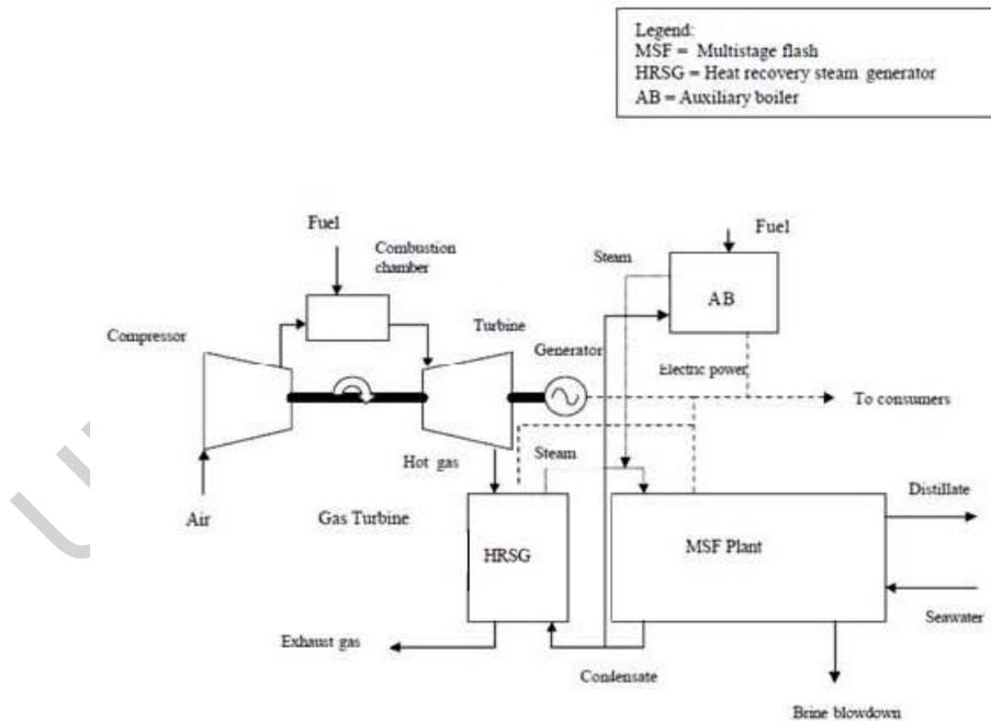
Figure 1 A conventional GT/HRSG/AB/MSF cogeneration plant (System 1)
