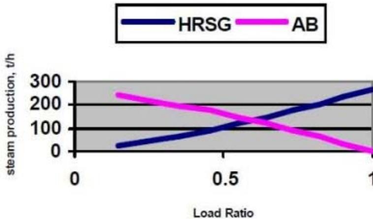
Figure 7 HRSG and AB steam productions at various GT load ratios
