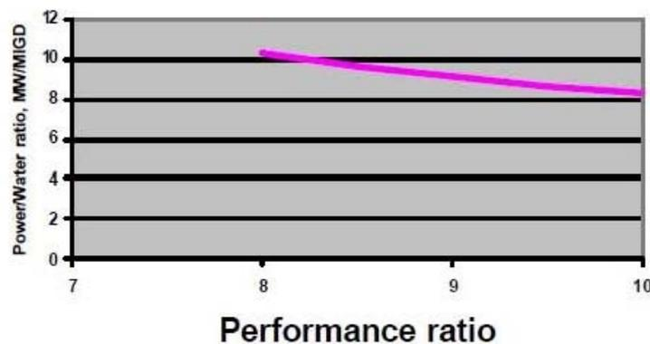
Figure 3 Power to water ratio and design capacity of MSF unit associated with a GT having a capacity of 100 MW
