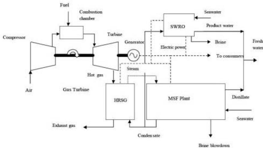
Figure 4 Improved GT/HRSG/MSF/RO hybrid cogeneration system (System 2)
