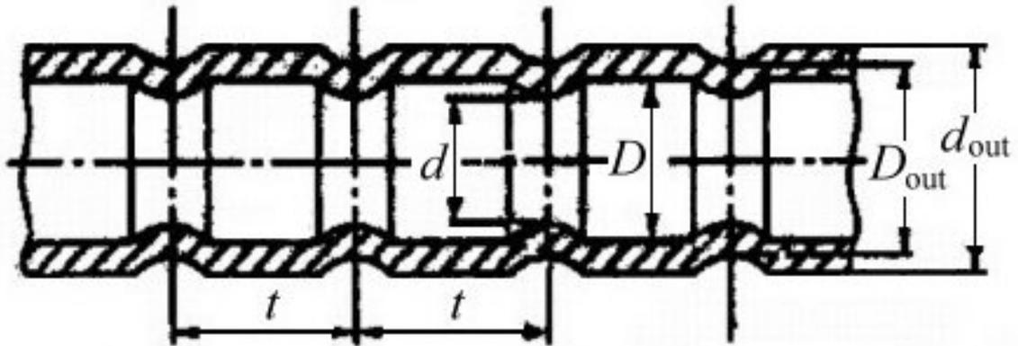
Figure 1. A tube with annular turbulators
