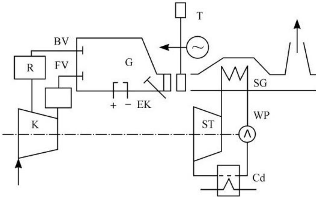
Figure 1: GTE with three-valved chambers, combustion at constant volume with the additional steam turbine (ST), water pump (WP) and condenser (Cd)
