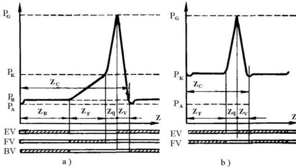
Figure 2: The temporal character of processes in GTE with three-valved chambers, combustion at constant volume with the additional steam turbine (ST), water pump (WP) and condenser (Cd)
