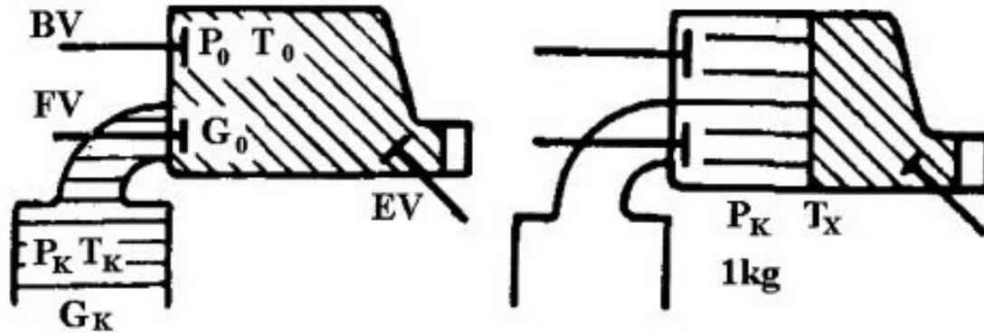
Figure 4: Filling and emptying of the chamber
