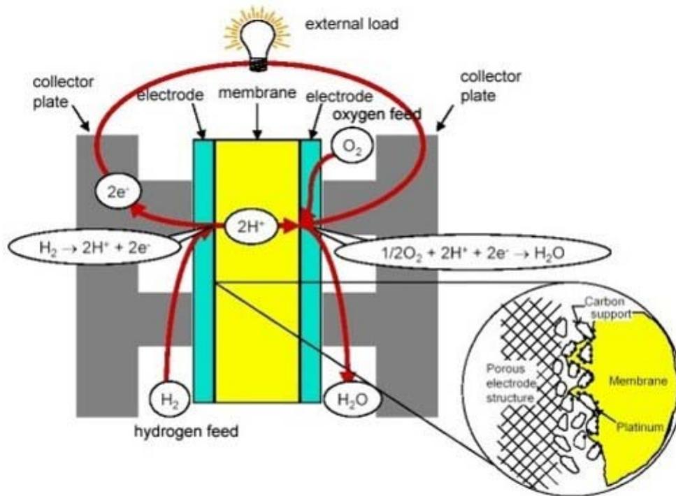
Figure 1. Schematic representation of a PEM fuel cell
