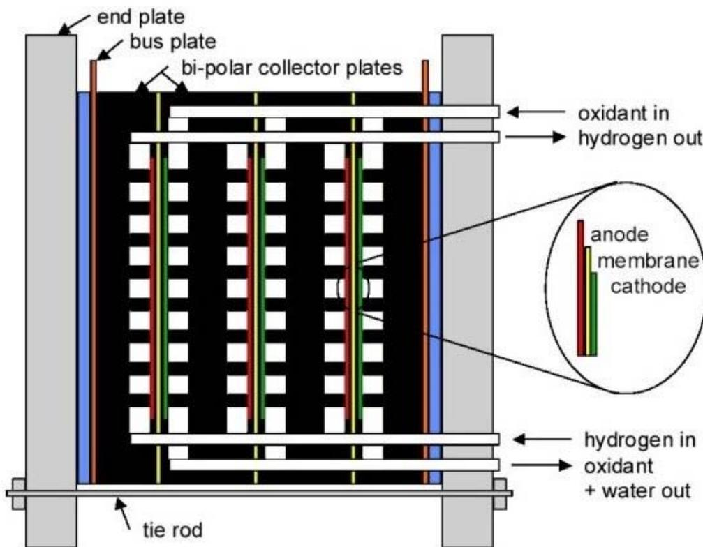
Figure 2. Schematic representation of a PEM fuel cell stack
