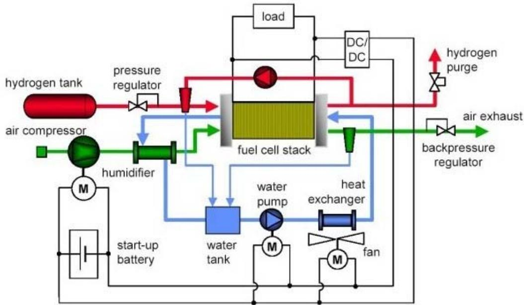
Figure 4. Schematic of an automotive fuel cell system
