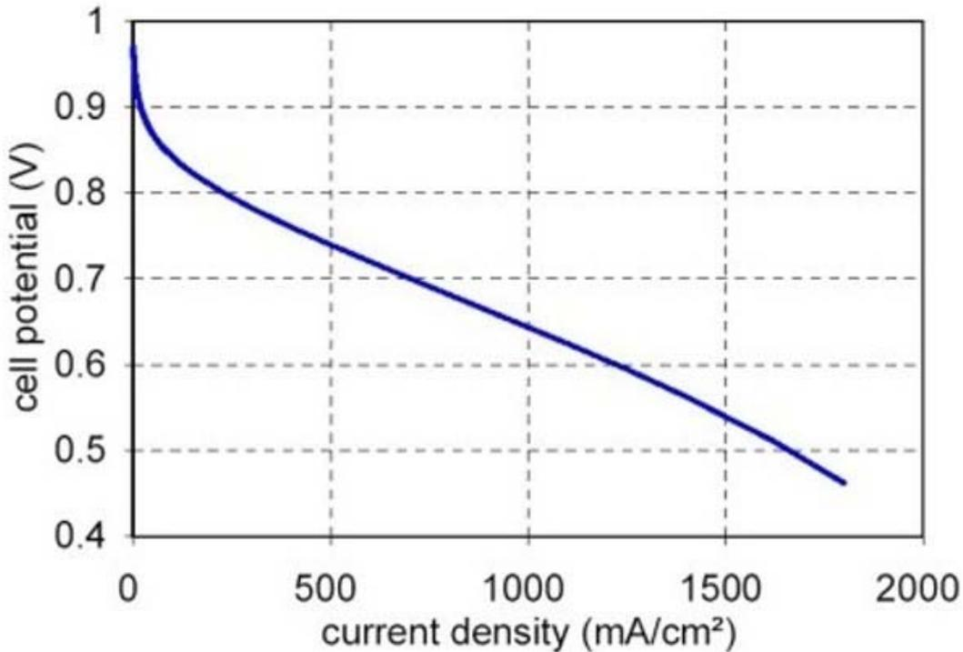
Figure 3. Typical PEM fuel cell polarization curve H<sub>2</sub>/Air; 3 bar, 60 °C
