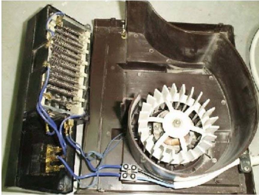
Figure 1: Typical power heater
