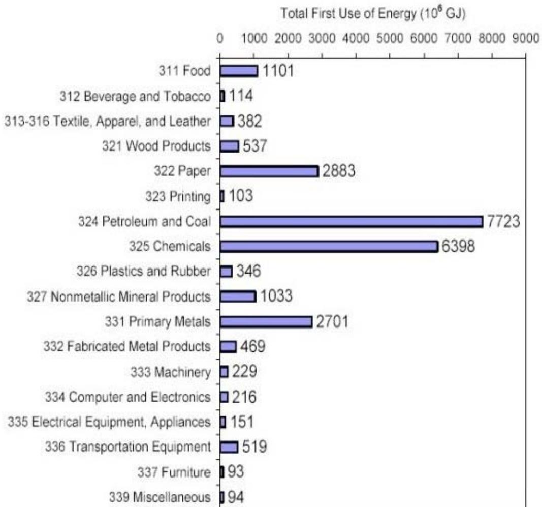
Figure 5. Total energy consumption by manufacturing industry, 1998 (United States)
