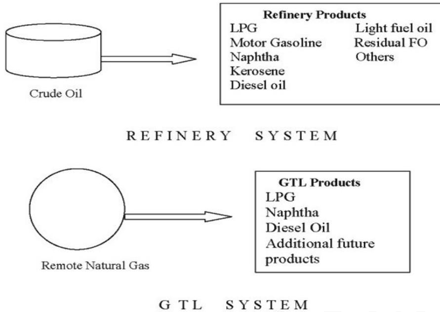
Figure 1. Comparison between Refinery Set-up and GTL System
