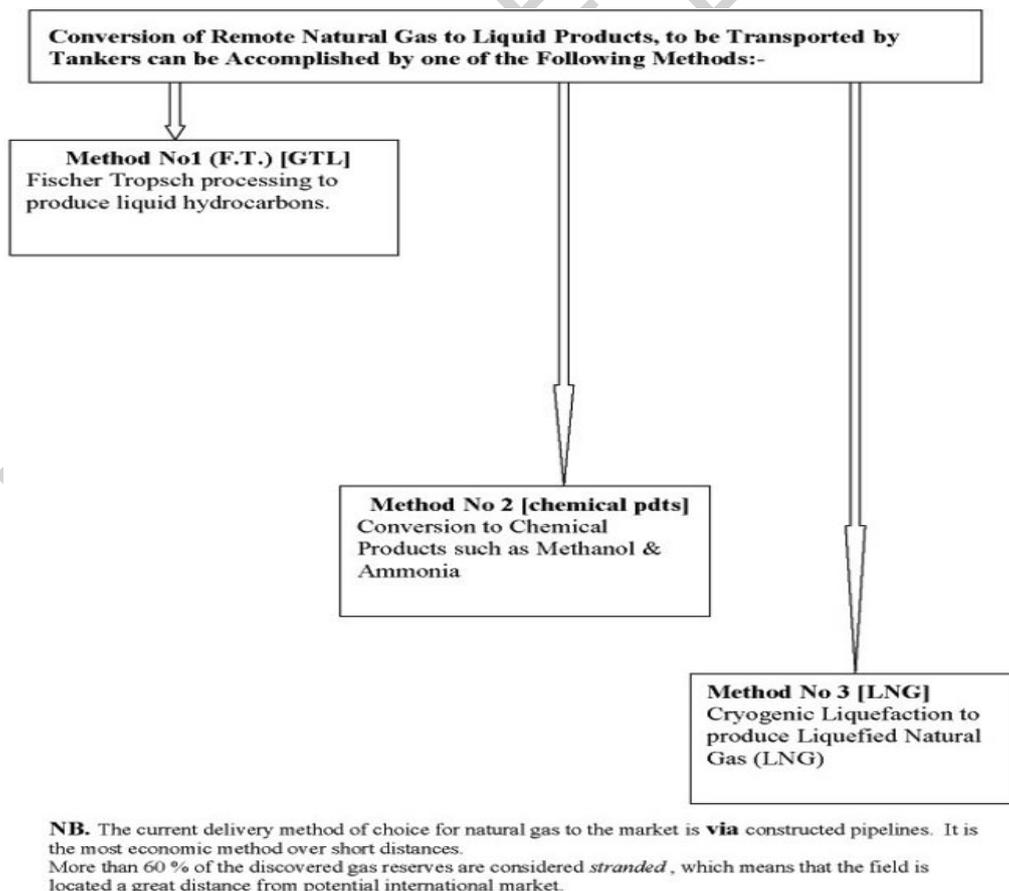
Figure 2. Options Available for shipping Remote Reserves of Natural Gas in Liquid Form
