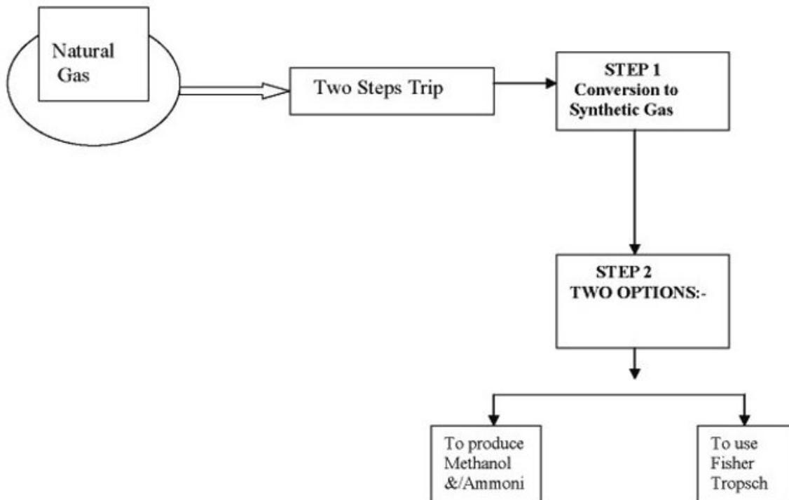
Figure 3. Current Approaches for GTL Technology
