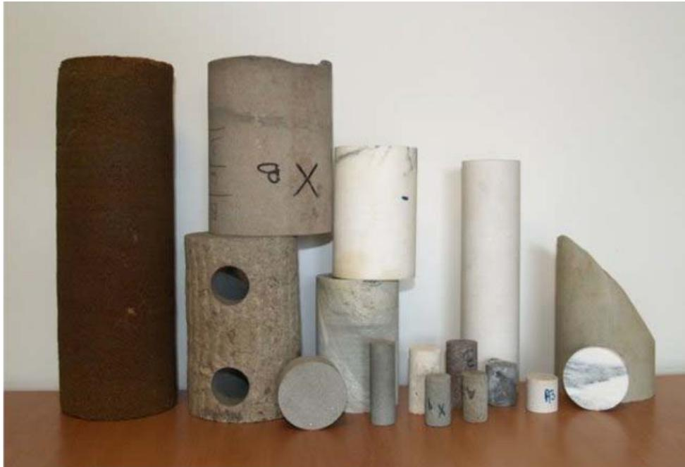
Figure 1. Full diameter core (left) and core plugs (right) cut for laboratory measurements. Cores can be full diameter cores (that is, they are nearly as large in diameter as the drill bit) taken at the time of drilling, or sidewall cores, generally less than 1 inch (2.54 cm) in diameter, taken after a hole has been drilled. Core plugs are cut from full diameter cores.
