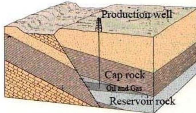
Figure 4. Reverse fault trap. (Picture courtesy of the Authors)
