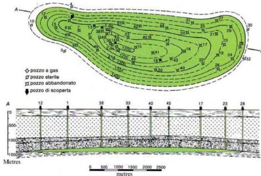
Figure 3. Hydrocarbon reservoir contained in a structural trap (anticline). The gas (green) is in contact with a bottom aquifer. (Caviaga gas field, Italy). (Picture courtesy of the Authors)
