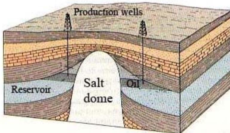
Figure 5. The intrusion of a salt dome, interrupting the continuity of the pierced strata, paves the way for the formation of geological traps. (Picture courtesy of the Authors)
