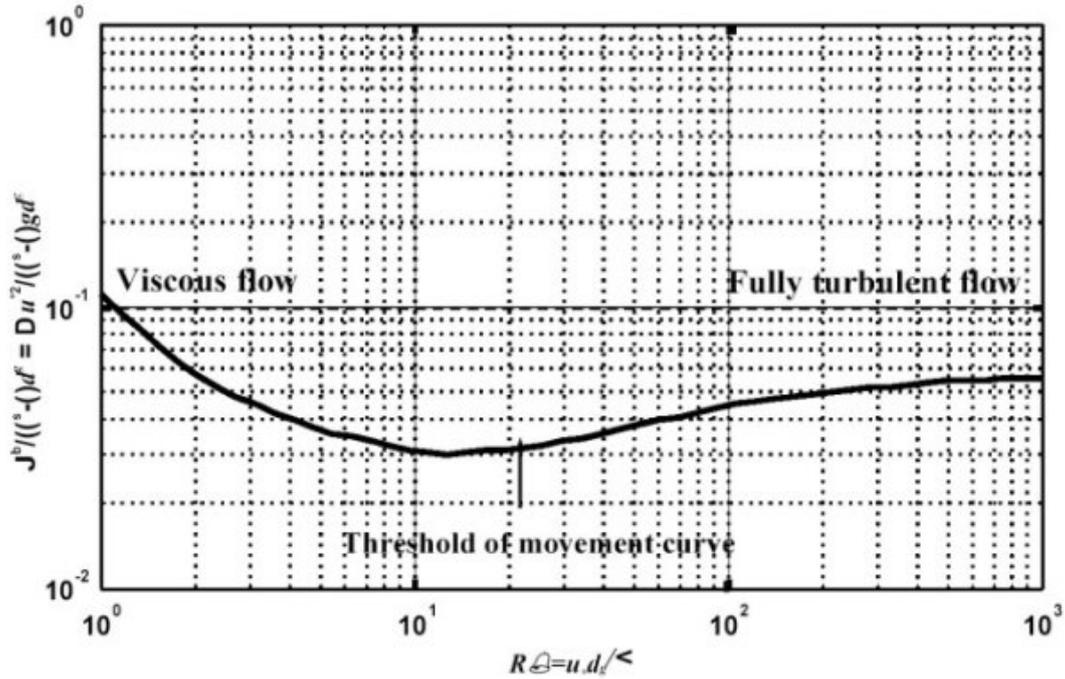
Figure 1. Shields Curve for incipient motion of cohesionless sediment
