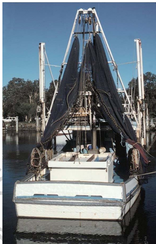
Figure 2. Modern prawn (shrimp) trawler from eastern Australia, with large deck working area
