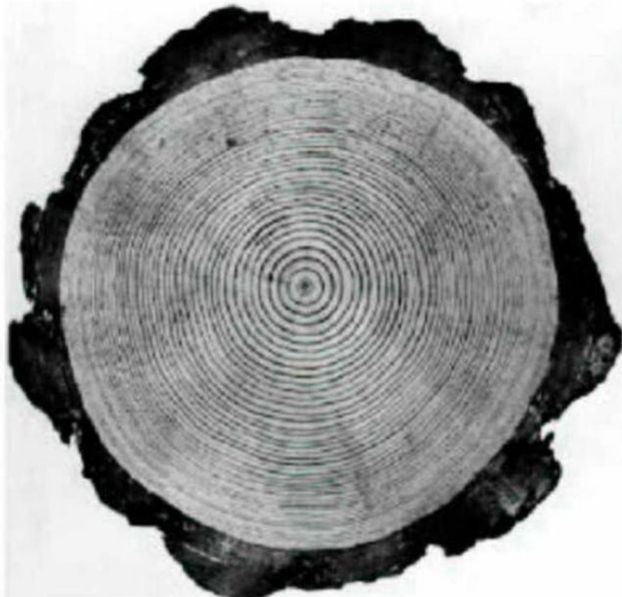
Figure 2. Cross section of ponderosa pine log showing growth rings. Light bands are earlywood and dark bands are latewood. A growth ring is composed of an inner earlywood zone and an outer latewood zone. (Forest Products Laboratory).
