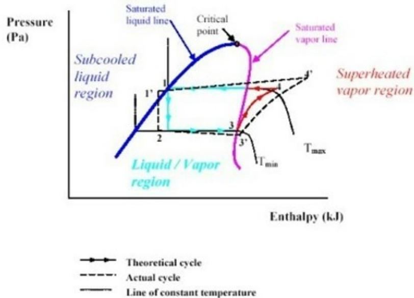
Figure 2. Simple compressible vapor Pressure–enthalpy diagram. ( $T_{\min}$ ) is minimum temperature, ( $T_{\max}$ ) is maximum temperature.
