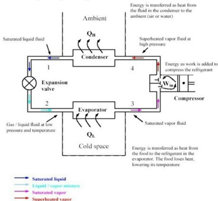
Figure 1. Diagram of a simple compressible mechanical vapor cycle. ( $Q$ ) is energy
