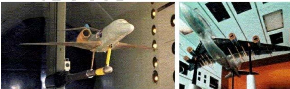
Figure 2: Wind tunnel tests on a scaled model of (a) a Cessna and (b) an Airbus A380.
