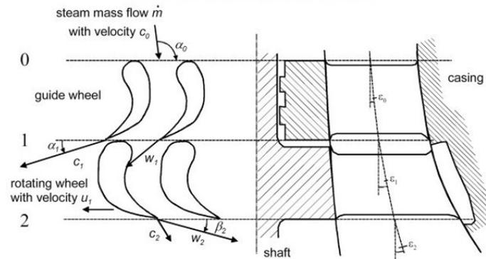
Figure 6. Guide wheel and rotating wheel.  $c_i$ : absolute velocities;  $w_i$ : velocities relative to the rotating wheel
