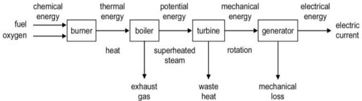
Figure 2. Energy conversion in a fossil-fuelled power plant
