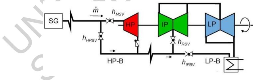
Figure 9. Turbine with HP and IP bypass station
