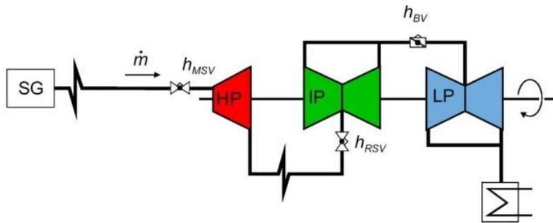
Figure 8. Reheating after the HP section
