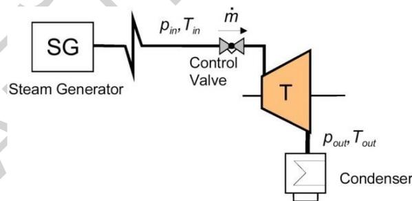
Figure 5. Steam flow through a turbine
