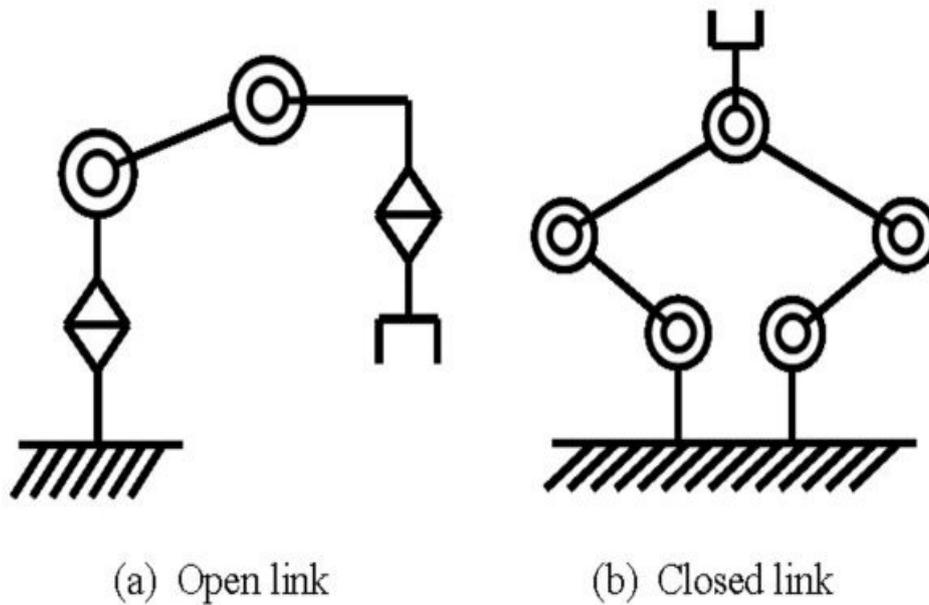
Figure 2: Link mechanisms
