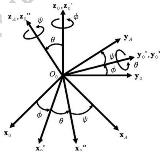
Figure 7: Representation of Z-Y-Z Euler angles.
