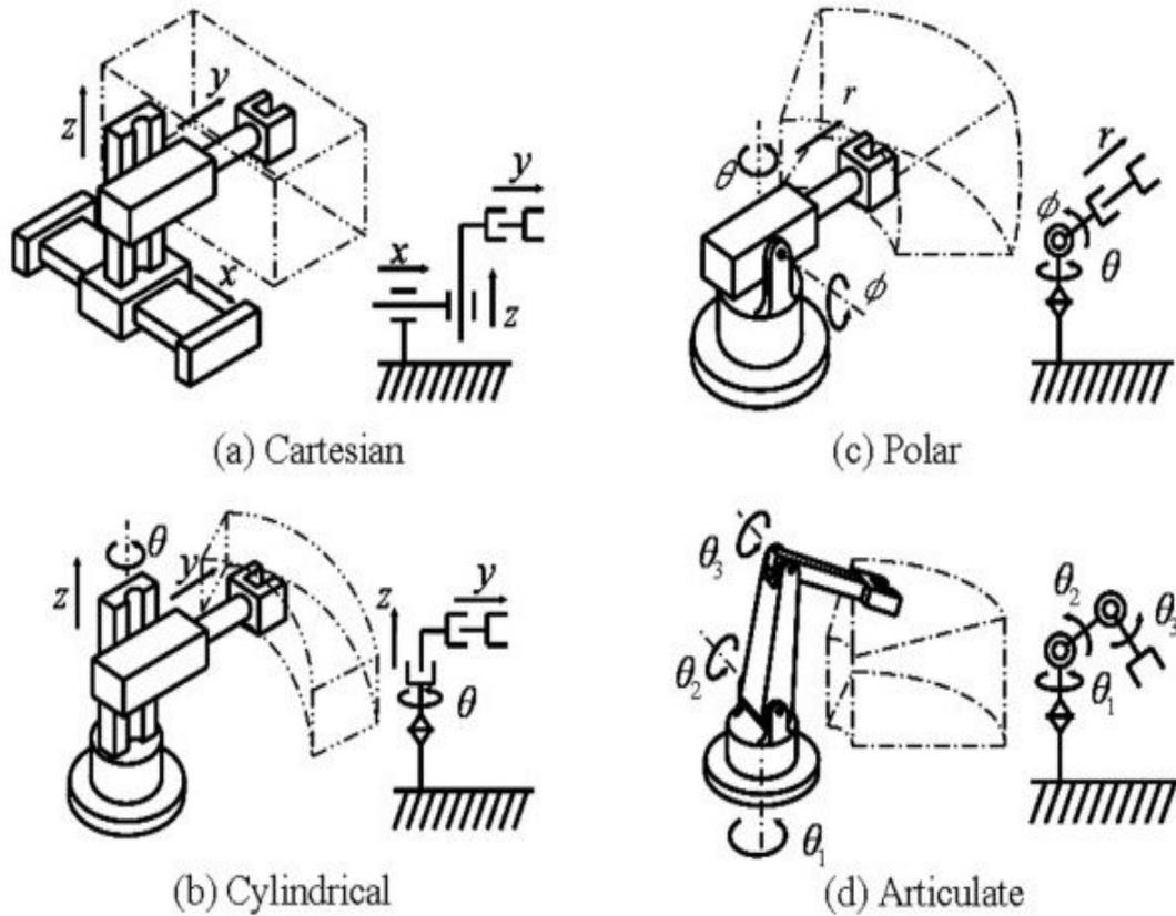
Figure 3: Robot configurations
