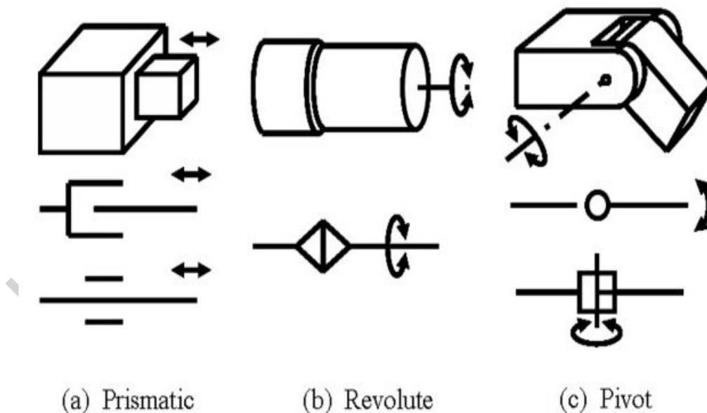
Figure1: 1 DOF joints and conventional representations
